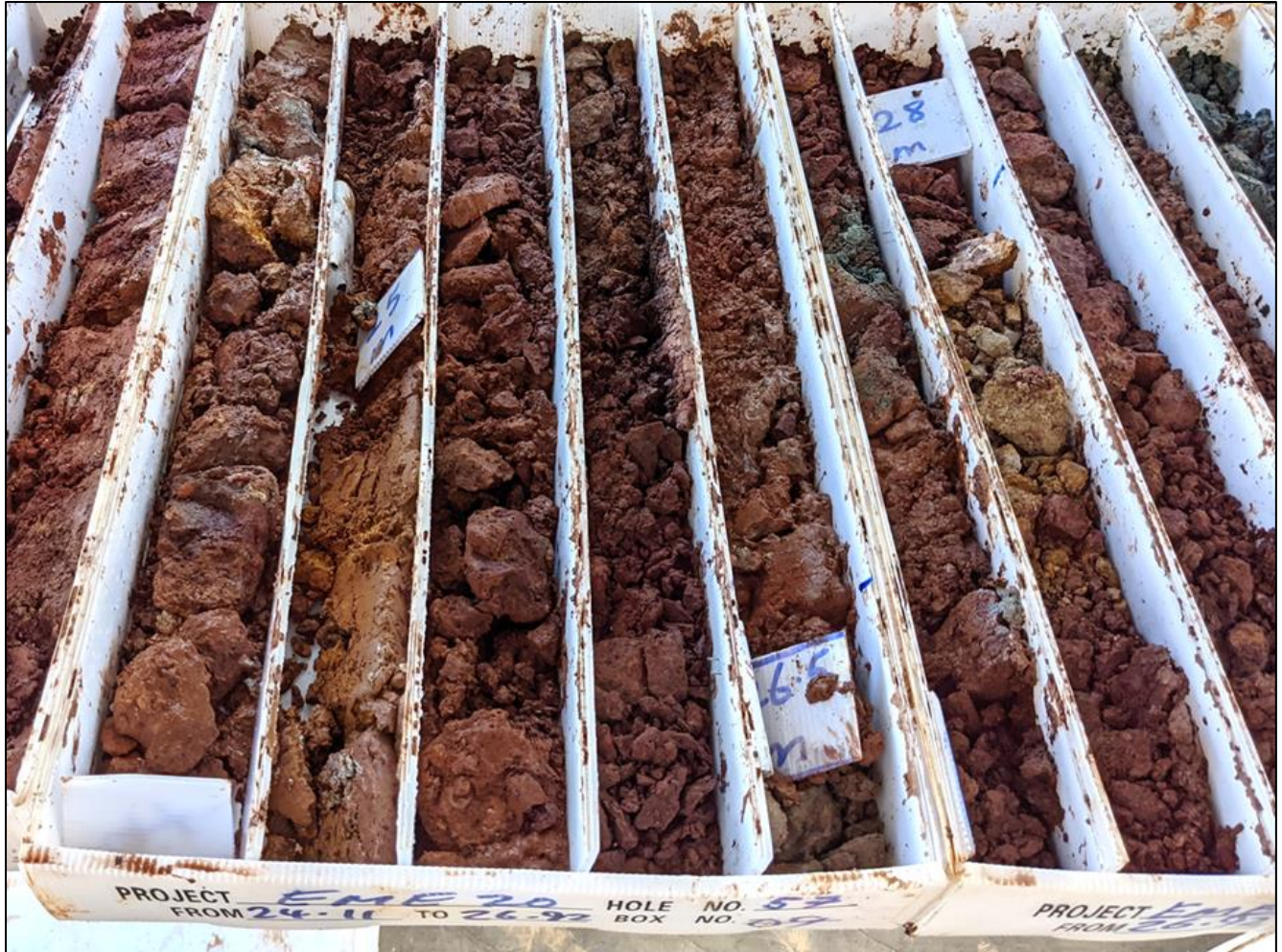
Figure 7-8: Typical mineralized saprolite core from the Salbora area in DDH EME20-57
