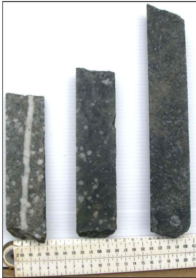
Figure 7-2: Host rock and alteration associated with molybdenum mineralisation
