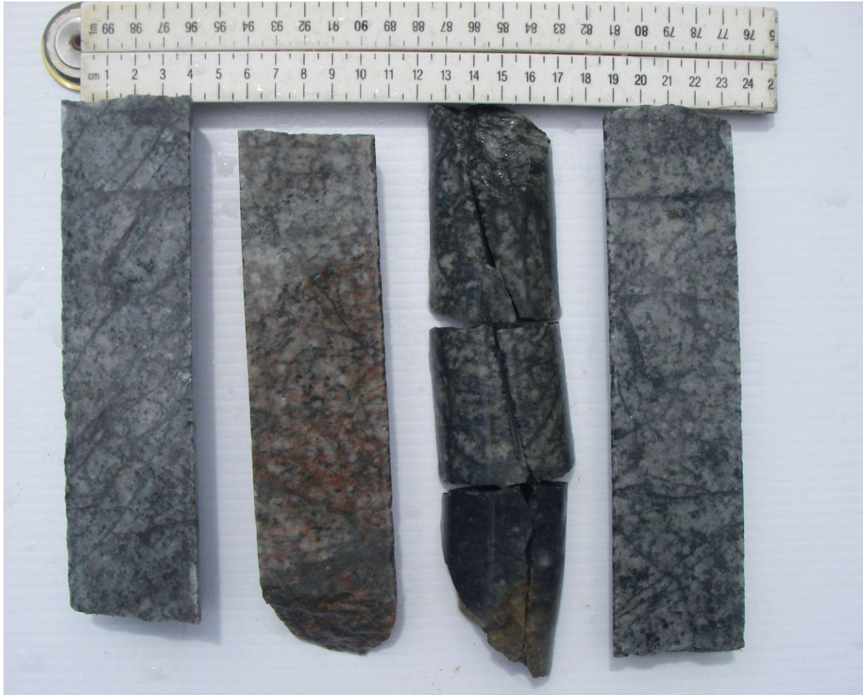
Figure 9-1: Characteristic mineralisation core photos: Saddle, Zion, Kilroy, Millionaire zones.
