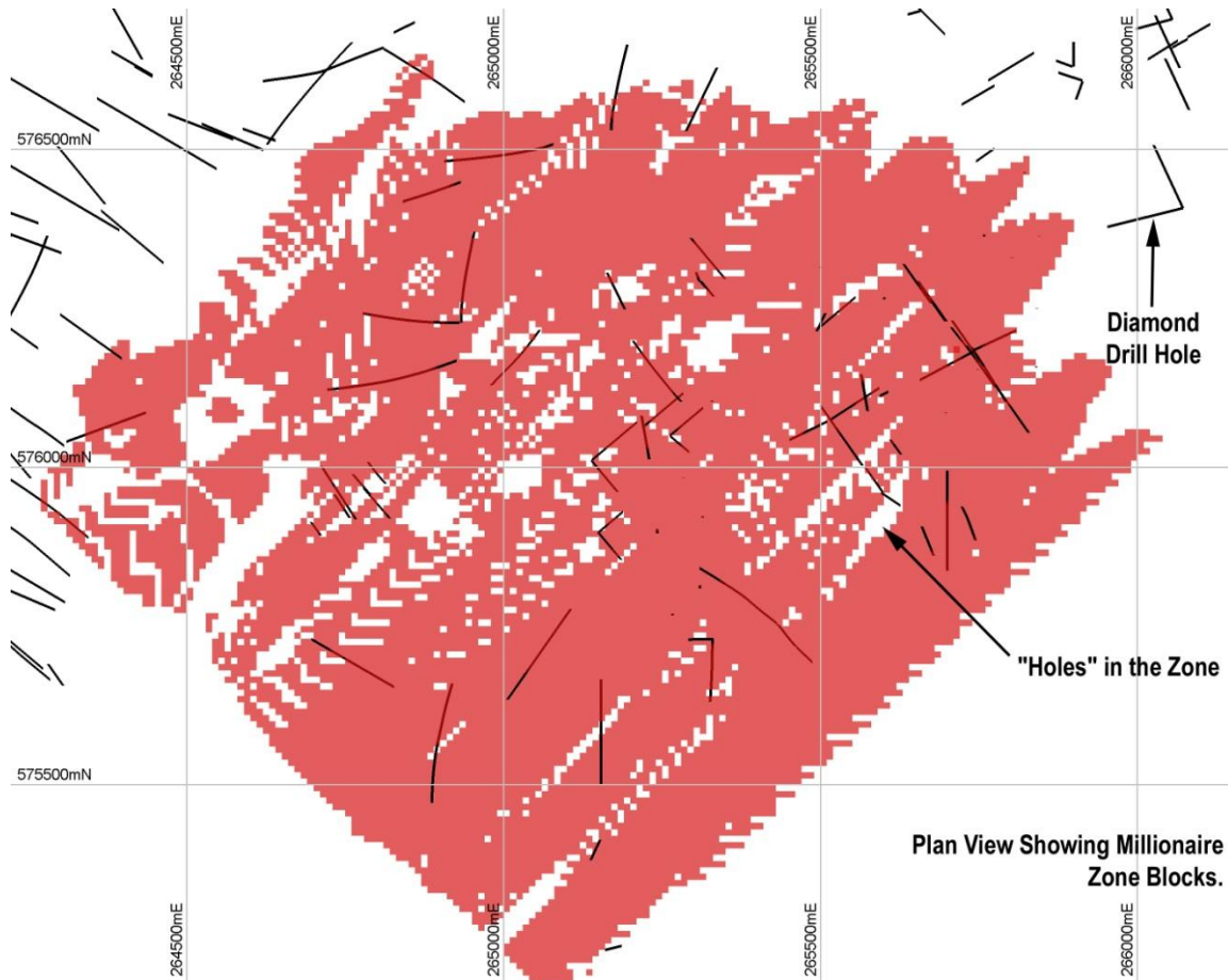
Figure 17-9: Plan view of Millionaire Zone block model showing gaps or holes in the model (ITS's "rock code" model).
