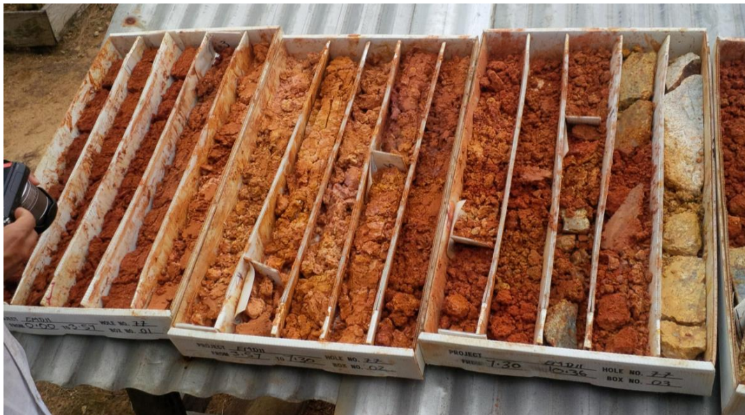
Figure 7-11: Typical Mineralized Saprolite Core in DDH EMD11-77.
